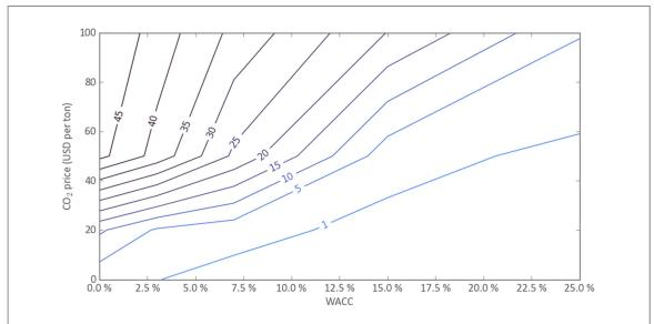
**Figure 5.** Contour-plot of renewable energy shares in percent. The colored lines show the combinations of discount rate and carbon price that trigger a specific renewable energy share in annual electricity generation.
