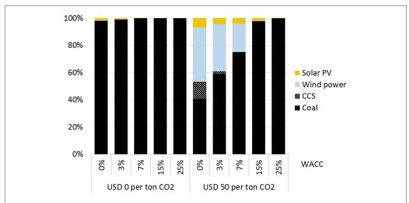
Figure 3. The generation mix for different capital costs and  $CO_2$  prices (natural gas assumed to be unavailable). As expected, higher  $CO_2$  prices and lower capital costs favor wind and solar power. A combination of a  $CO_2$  price of USD 50 per ton and low capital costs is required to push the share of unabated coal below 50%. See supplementary figures S1 and S2 for sensitivity analysis on carbon prices and natural gas availability.
