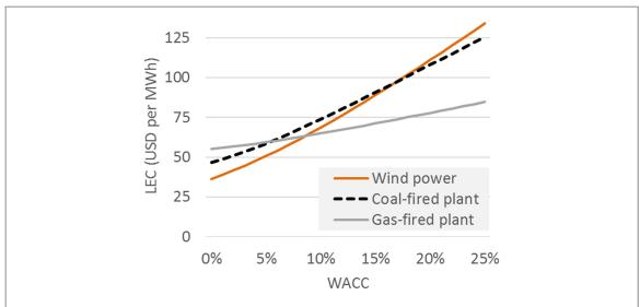
**Figure 2.** Generation costs of coal-fired, natural gas-fired, and wind-propelled plants for different WACC. Wind power levelized electricity costs (LEC) are the most sensitive to the cost of capital, because the share of upfront-costs is highest. Under these cost assumptions, wind power is the least-cost power source for WACC below 8%, but not at higher capital costs.
