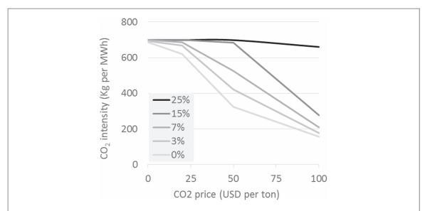
Figure 4. Carbon intensity of power generation.  $CO_2$  emissions are almost completely insensitive to carbon pricing if capital costs are high (WACC of 25%). The lower the capital costs, the more the emissions decline as a response to the same carbon price.
