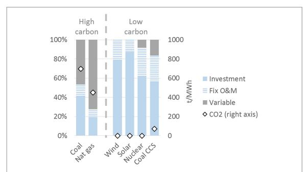
**Figure 1.** Cost composition of different power generation technologies. Typical parameters were used: 7% WACC and capacity factors of 60% for fossil fueled plants, 35% for wind power, 20% for solar power, and 90% for nuclear. A price of USD 30 per t  $CO_2$  was assumed. Under these assumptions, the levelized electricity costs of all technologies are comparable in level (USD 58–84 per MWh).
